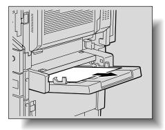
2 If misfed paper cannot be pulled out, pull the lever for the sliding plate of the bypass tray, and then pull the sliding plate toward you.
